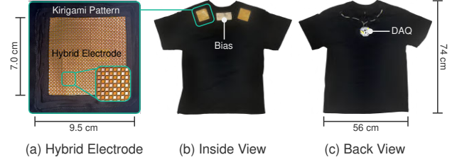
Figure 4: Implementation of the proposed system. (a) Hybrid electrode integrated into a stretchable kirigami pattern. (b) Inside view of the prototype showing two sensing electrodes and the central bias electrode. (c) Exterior back view showing the data acquisition system (DAQ).
